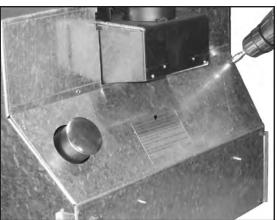
Figure 47: Removing Back Plate From Sonnet.
